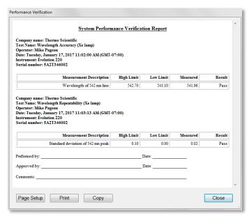
4. If all tests pass, no further actions are required. If any tests fail, the Evo220 will need to be calibrated using the Xenon lamp. See below for further instruction.
